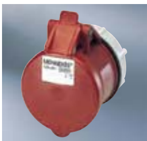
▲ IP 44 CEE panel mounted receptacles RAPIDO with central locking system and screwless TwinCONTACT, round flange for central fixing, dia. 70 mm Dim.: page 60/61
