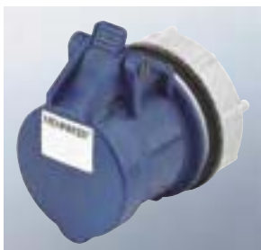
▲ IP 44 CEE panel mounted receptacles, RAPIDO with central locking system and screwless TwinCONTACT, round flange for central fixing, dia. 61 mm Dim.: page 60/61
